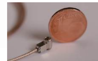
Indirect action sensors: Sensors for use under the ejector pin by BAUMER of Switzerland
